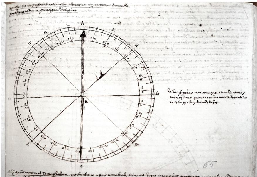
FIGURE 3 Allacci's copy of Stevin's first instrument with a marginal note on how to divide the degrees
